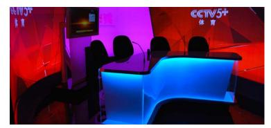
The small Internet studio was designed by Mark Dyson with a desk as the focus point. Using 20mm Clear Perspex<sup>®</sup> sheet we manufactured a clear outer case to complete the desk and enhance the LED features.
